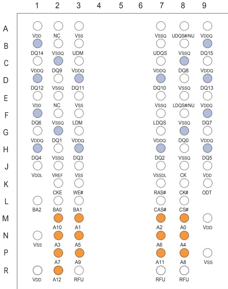
Figure 1: 84-Ball FBGA - x16 Ball Assignments (Top View), 1Gb, HW
